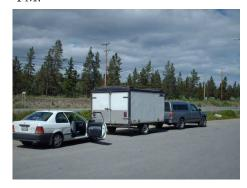
Due to the fact that our 12' trailer was filled heavily with only one axle and passenger rated tires instead of more sturdy trailer tires, we had difficulty keeping it from fishtailing behind our truck. After a few days we stopped and replaced the tires and also added a weight-distributing hitch. These improvements created a much more pleasant drive.
